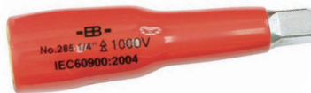
WIH12854 1/4" X 50 MM · Insulated 1000 Volt Rated 10,000 Volt Tested · Meets ASTM F1505, EN/IEC 60900, NFPA-70E · Additional Durable Soft Grip
